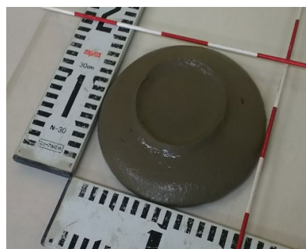
写真-1 流動化処理土 Photo.1 Fluidized soil-cement mixture
