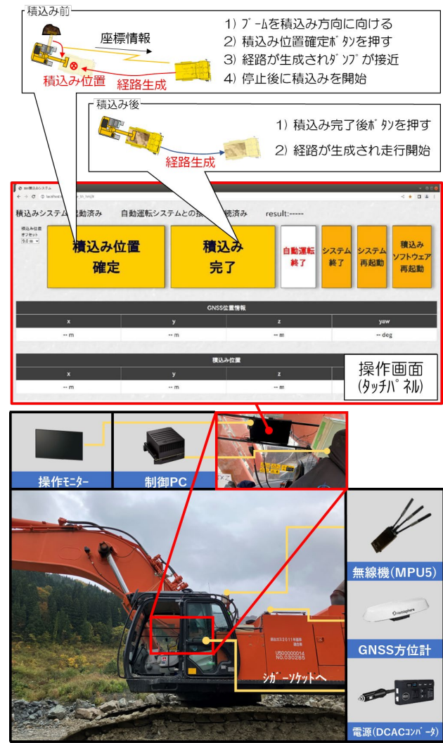
図-4 T-iROBO Rigid Dump の外観及び搭載機器 Fig.4 Appearance and on-board device of T-iROBO Rigid Dump
