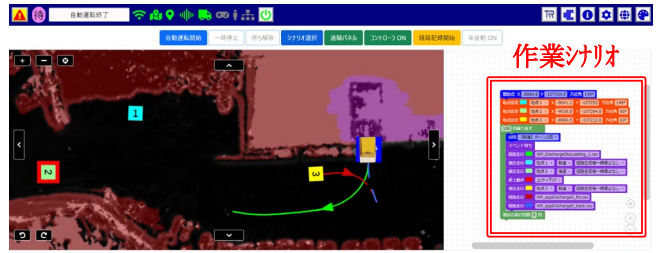
図-5 T-iROBO Rigid Dump の操作画面 Fig.5 Screen operation system of T-iROBO Rigid Dump
