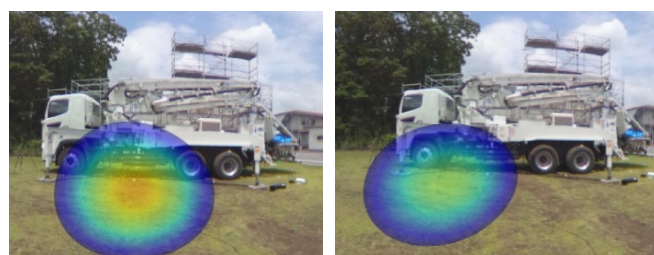
図-7 音源探査結果 高圧圧送時 (左：S13 500 Hz 帯域, 右：S13 1000 Hz 帯域) Fig.7 Noise source identification results during high-pressure pumping (left: S13 500 Hz band; right: S13 1000 Hz band)
