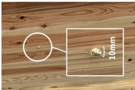
写真-4 先孔追い加工時の失敗事例 Photo.4 Examples of Failures during Predrilling
