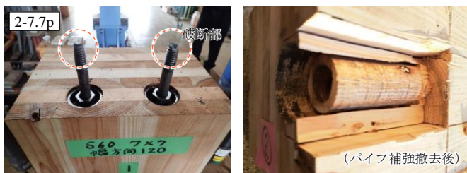
写真-2 LSB 接合部の破壊性状 Photo.2 Failure behavior of LSB joint
