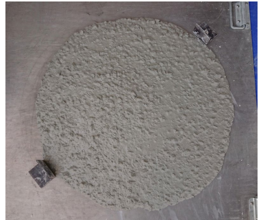
写真-5 Carbon-Recycle の広がり状況 Photo.5 Slump flow spread of Carbon-Recycle
