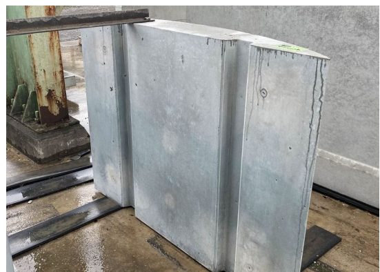
写真-7 Carbon-Recycle の脱型後外観 Photo.7 Condition after invert demolding
