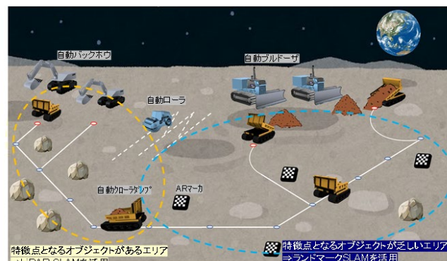
Fig.6 SLAM autonomous driving using AR markers 7)
