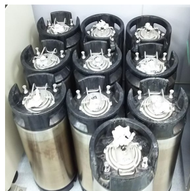
写真-2 耐圧培養容器を用いた UCH007 株の大量培養 Photo.2 Mass cultivation of strain UCH007 using pressure-resistant vessels
