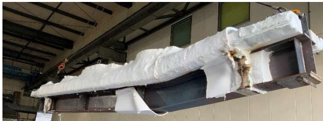
写真-5 載荷加熱後の試験体 Photo.5 Specimen after load heating
