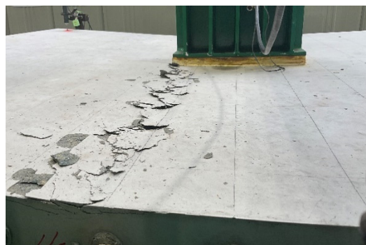
写真-4 終局後の試験体上面 Photo.4 Top surface of specimen after failure
