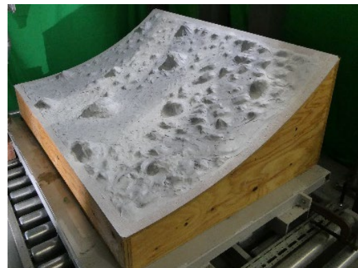
図-8 模擬地盤面 Fig.8 Artificial uneven ground
