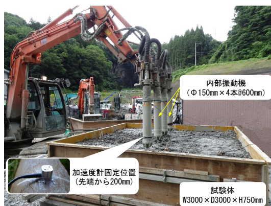
写真-1 累積エネルギーの計測状況 Photo.1 Accumulated energy measurement status
