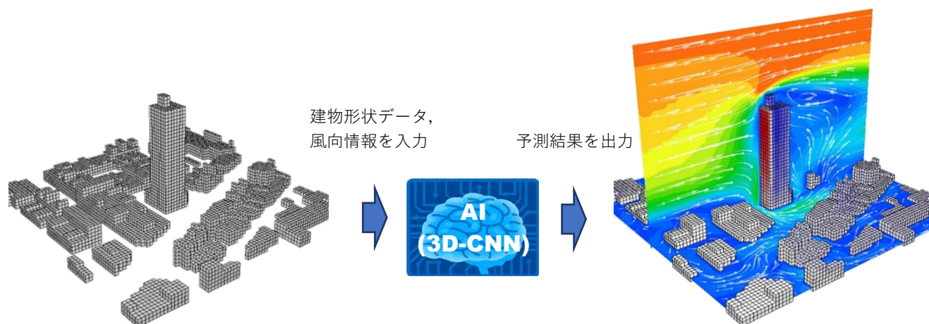
図-1 AI技術を用いた風速・風圧分布予測の概略 Fig.1 Outline of prediction of wind velocity and pressure distribution using AI
