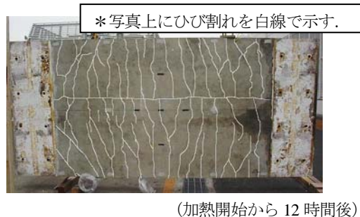
写真-1 試験体裏面のひび割れ状況 Photo. 1 Crack on back side of specimen
