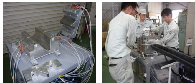
図-17 現場接続用圧着機(左)および性能確認試験(右) Fig.17 Joint tool (left pic.) and Handling test (right pic.)
