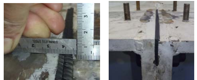
図-7 上蓋接合部段差(3mm)設定状況 Fig.7 Difference in joint of upper plates
