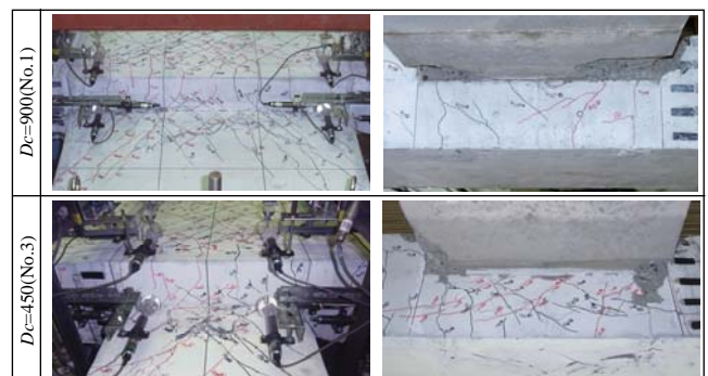
図-6 柱梁接合部直交面破壊状況 Fig.6 Crack pattern on side surface of beam-column joint
