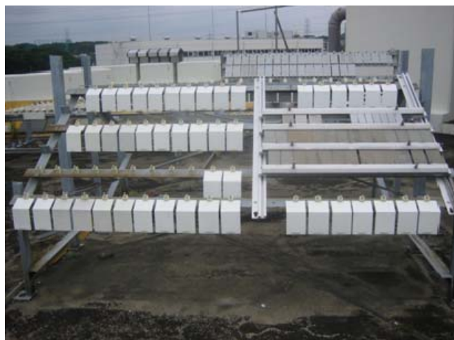
写真-2 塗料試験体の暴露状況 Photo2 Outdoor exposure test of coatings
