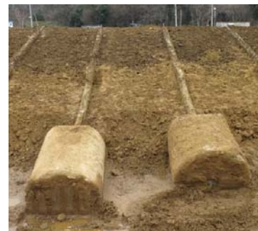
図-11 改良体(左:No.1 右:No.3) Fig.11 Improved soil column
