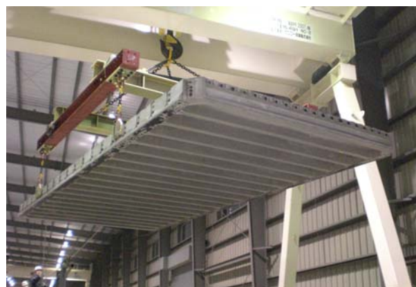
写真-8 UFC床版 Photo 8 UFC slab
