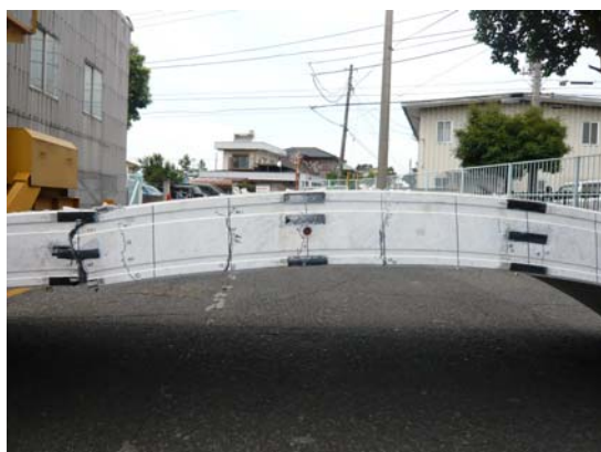
図-16 等曲げ区間ひび割れ発生状況（局所載荷終了時） Fig.16 Crack patterns of section of uniform bending moment
