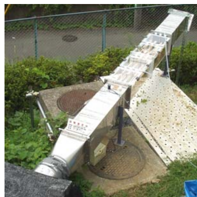
図-3 NO x 除去試験状況 Fig.3 NO x removal test situation
