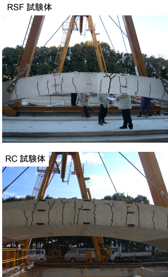
Fig.5 Crack patterns of test specimens
