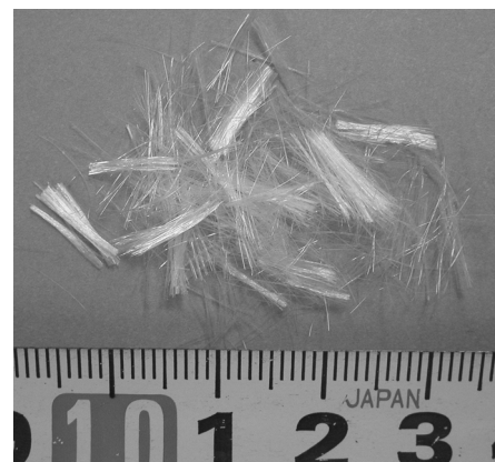
写真-1 爆裂対策用有機繊維 Organic fiber used for improving spalling resistance of high-strength concrete
