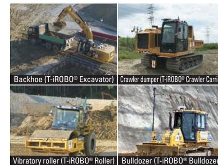
\*1 Unmanned construction technology: T-iROBO® series
